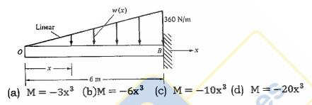
23. Consider the beam shown in figure. The beam is simply supported at its left end A and fixed at its right end B. It carries a load that varies in intensity from zero at support A to 'w' at support B according to the relation  $w_x = (x/L)w$ . The reaction component at A is
