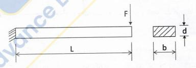
(a) The beam section has a uniform shear stress,  $\frac{F}{bd}$
