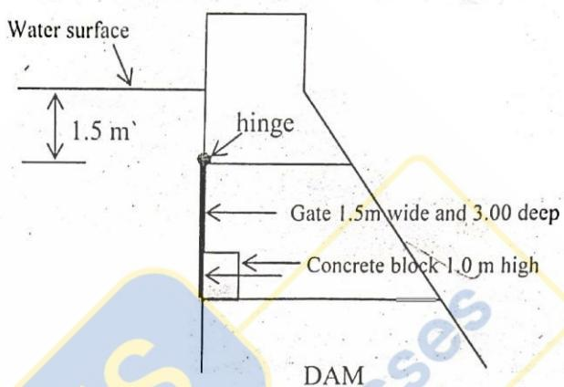
87. At what depth from the surface of water the centre of pressure is located ?
